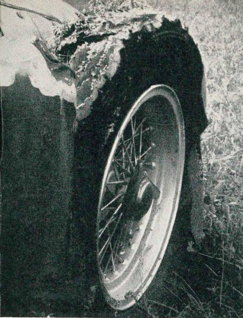
Used Tyre. The result of an Englebert tyre bursting on the Monza banking at high speed.
